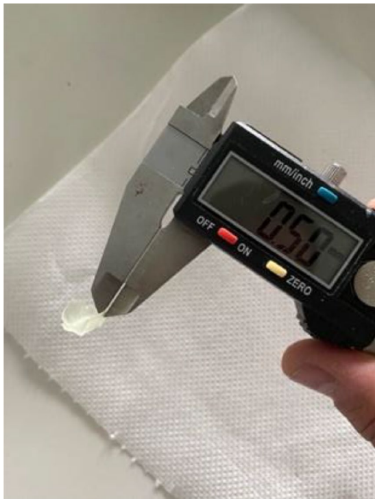
Fig. 1 Measured thickness of the aligner (0.5 mm) coinciding with the thickness designed in the CAD software
