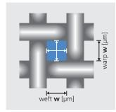
Mesh opening w [µm] The mesh opening w is the distance between two adjacent warp or weft threads.
